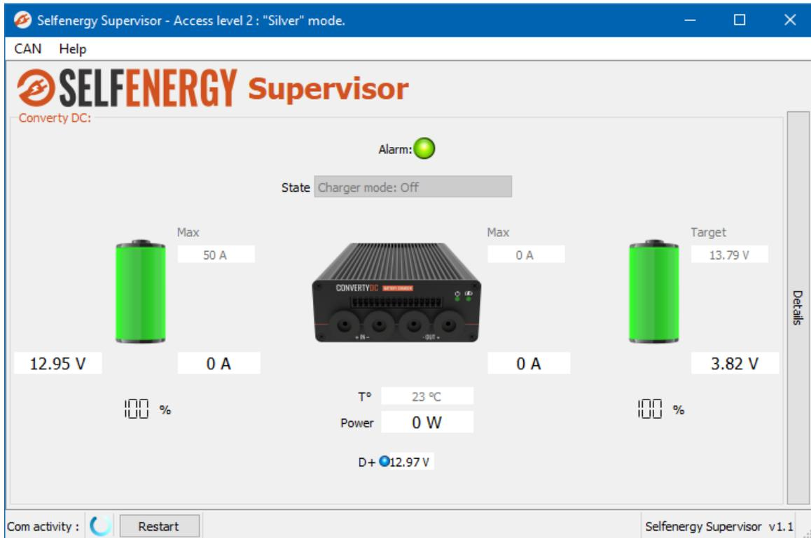
Figure n°9 : Supervisor's main panel in Silver mode
