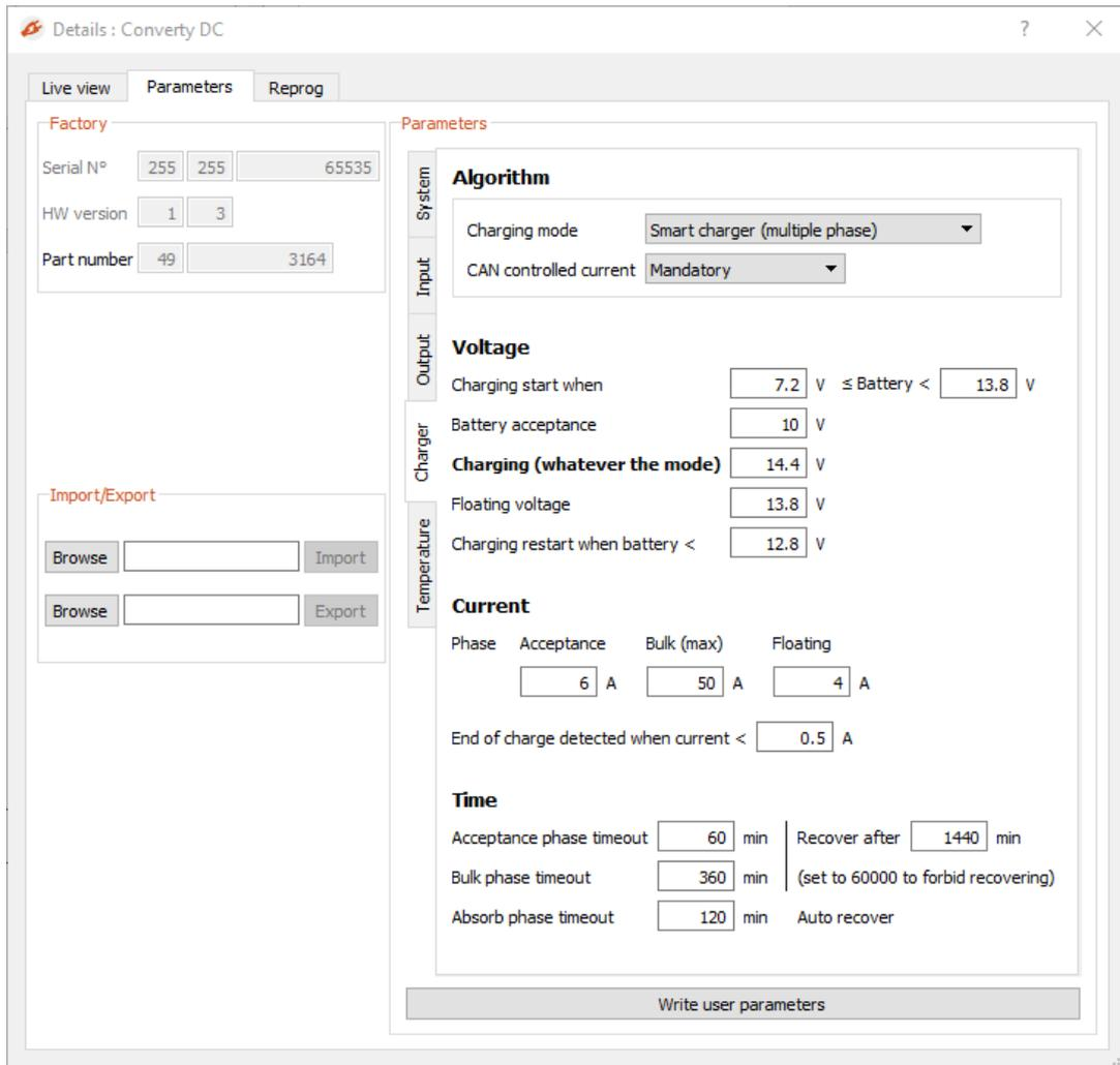
Figure 15 :Details window, “Parameters” tab in “Gold” mode
