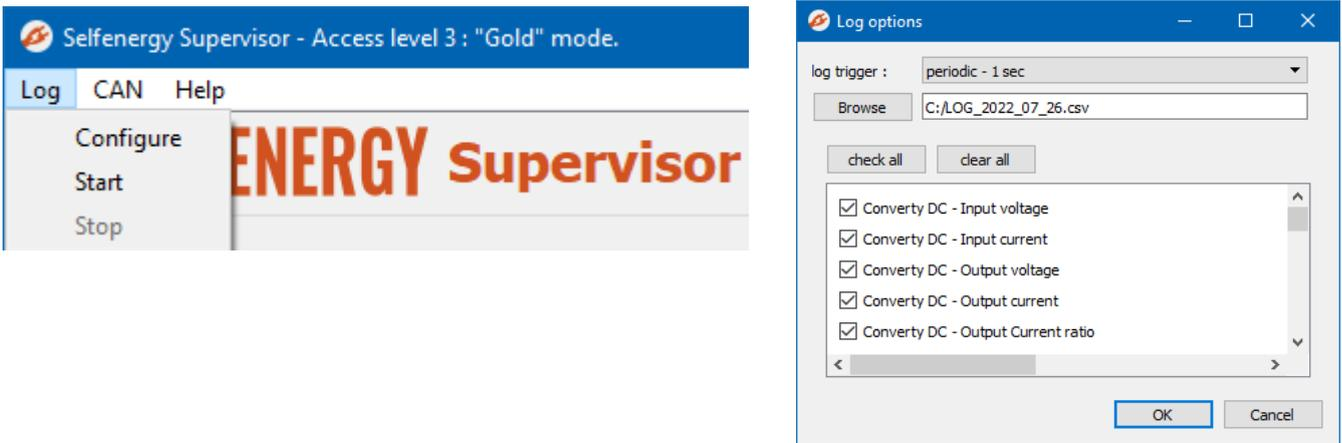
Figure 13 : Log menu and its configuration window
