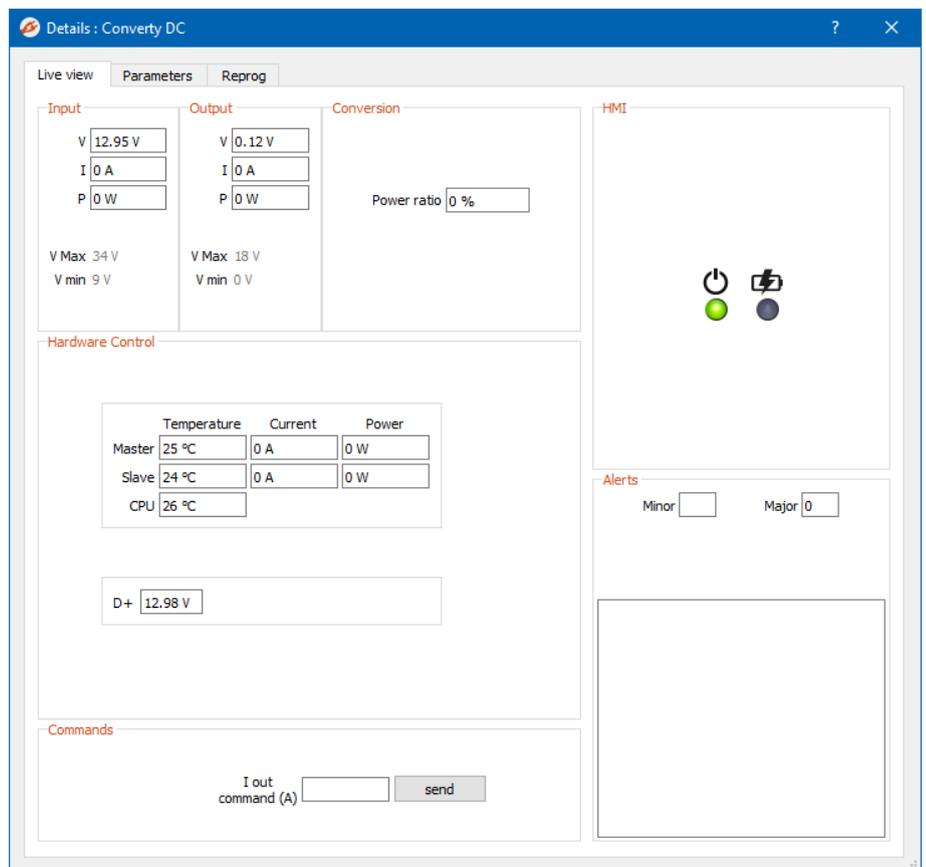
Figure 14 : Details window, "Live view" tab in "Gold" mode
