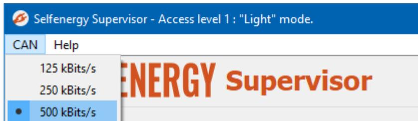
Figure 8 : CAN Baudrate choice in the Main window
